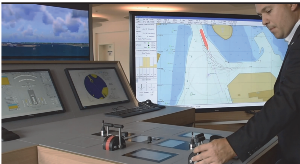
Fig. 5 Manoeuvring Monitoring & Conning Module – Demo of using bridge handles in to train “Touch and Feel” for Controls with Multiple Dynamic Prediction showing the effect of any control change immediately as future ship shape on ENC (SAMMON Demo on Bridge Simulator at benntec / Marinssoft Office at Rostock-Warnemünde Germany)
